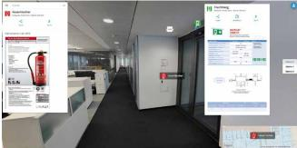
After the digital data has been transferred to a digital twin (3D point cloud model), the execution statuses can be mapped and shown in a walk-through virtual real image model.
