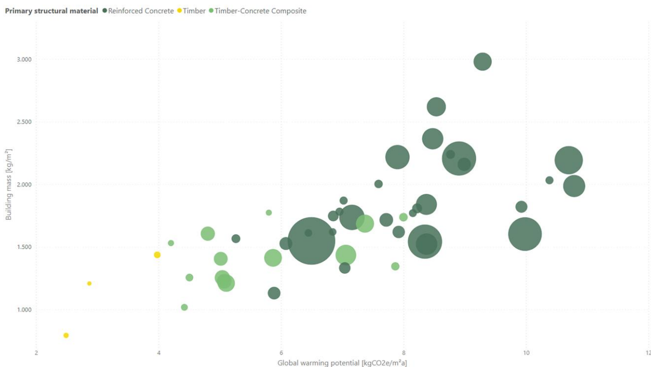
Figure 8: Representation of the sample by mass per NRF [kg/m 2 ] and GWP per NRF and year [kgCO 2 e/m 2 a]. Coloring by material of the primary supporting structure and size of the points by NRF of the building.
