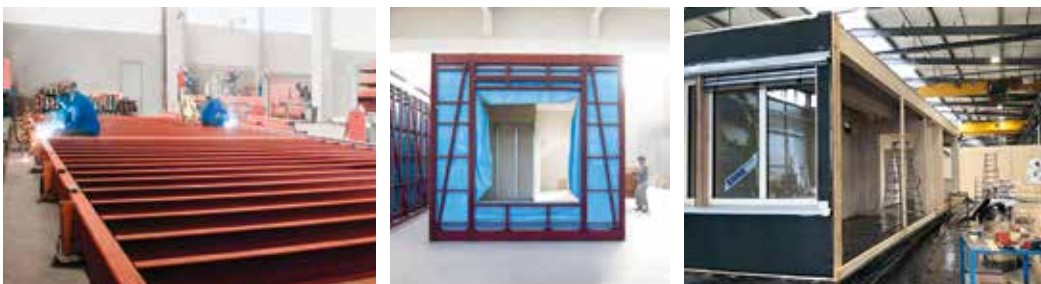
Fig. 9: Room modules in steel (left and middle: ADK) and wood (right: Erne)
